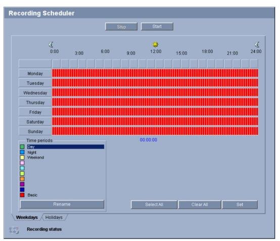
The recording scheduler allows you to link the created recording profiles with the days and times at which the camera's images are to be recorded in the event of an alarm. You can link any number of 15-minute intervals with the recording profiles for each day of the
